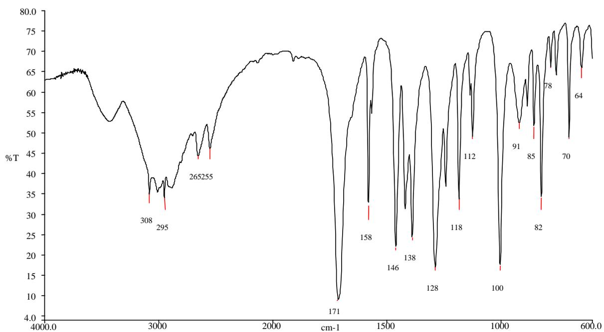
**Fig. 11** Infrared spectrum of dicamba
